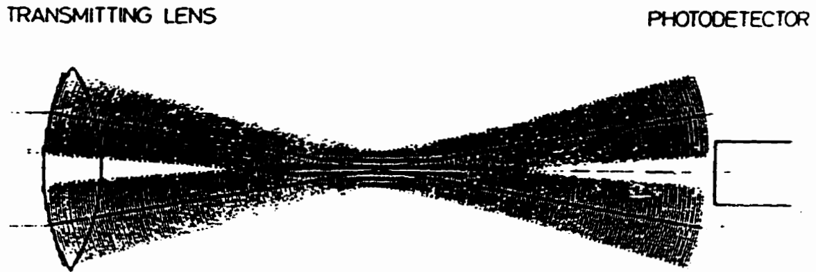
a) crossing of the beams at the beam waist
