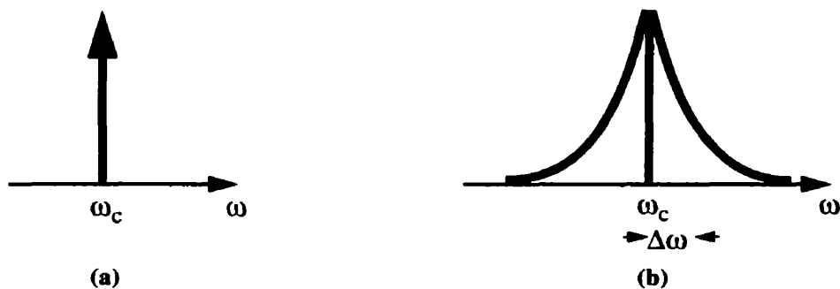
FIGURE 2.14 a) Output Spectrum of Ideal Oscillator. b) Spectrum of Actual Oscillator.
