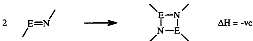
Figure 2.8. Cyclo-dimerization reaction of multiply-bonded compounds.
