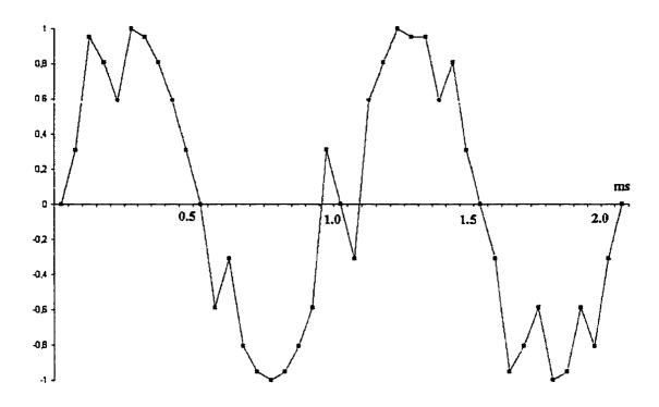
Figure 6. The digitized sinusoidal 1000 Hz tone is jittered by displacing several sampling points. Using this technique, distortion can be introduced to a digitized sound.
