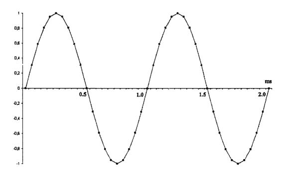
Figure 5. A sinusoidal 1000 Hz tone is digitized on a sampling rate of 20000 Hz. The dots mark the sound samples drawn from the continuous tone.
