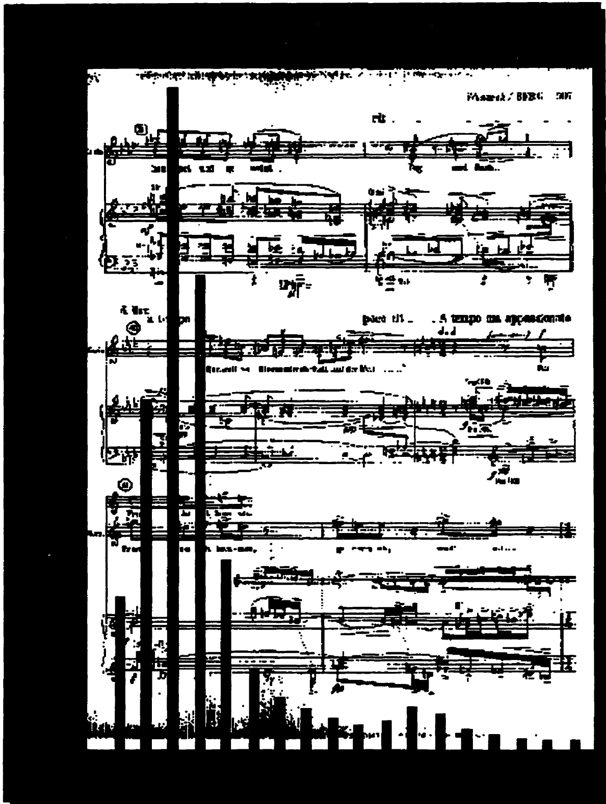
Figure 4.6 Estimating staffline_height by vertical black runs. The graph shows that the staffline_height of 4 pixels is most prominent.
