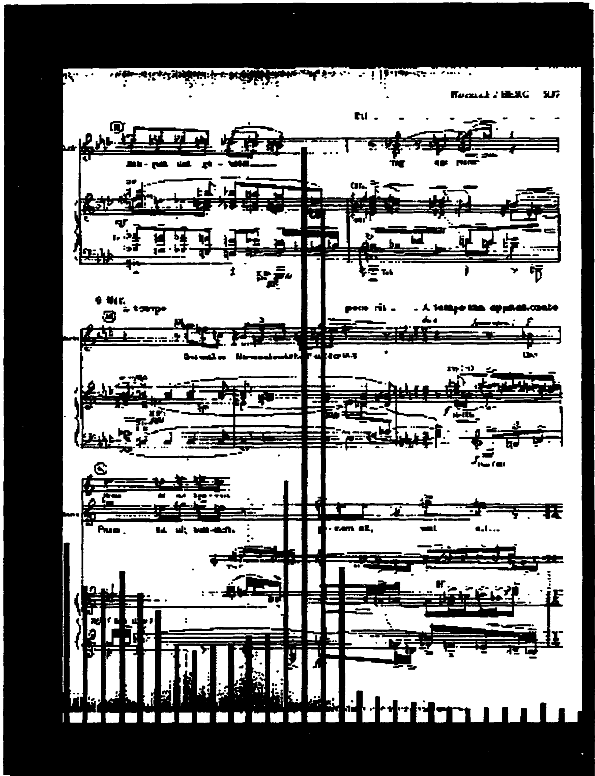
Figure 4.7 Estimating staffspace_height by vertical white runs. The graph shows that the staffspace_height of 14 pixels is most prominent.
