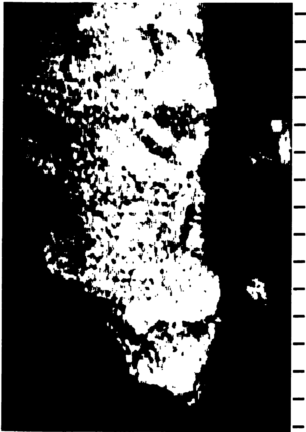
Figure 41. Image of a gravity current flowing along the top of the roughness elements showing the circulation generated within a roughness element space leading to mixing between the ambient and current fluids. Roughness element height = 2.5 cm. Source fluid density excess = 0.01. (Scales are divided in 1 cm increments. Roughness elements added graphically.)
