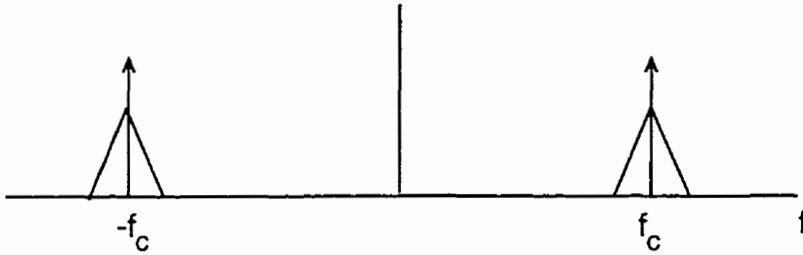
Figure 2.1. Narrowband bandpass signal
